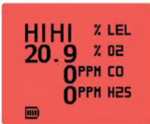
Red display in alarm conditions
