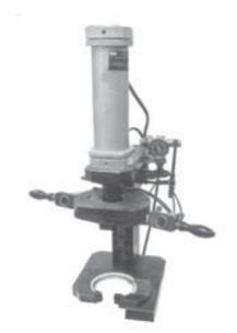
Loosening/tightening device for bayonet lock bezels
