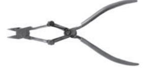
Adjusting pliers to close the pull rod eye
