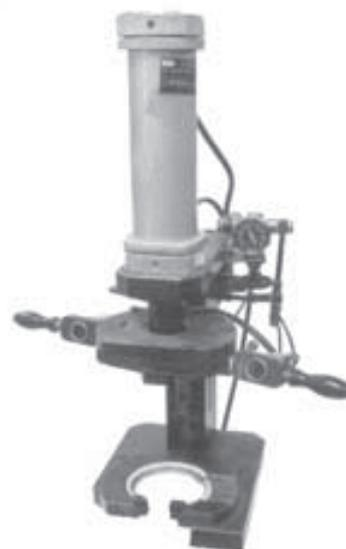
Loosening/tightening device for bayonet lock bezels
