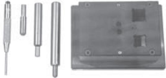
Tool set for driving rivets in and out to replace dials
