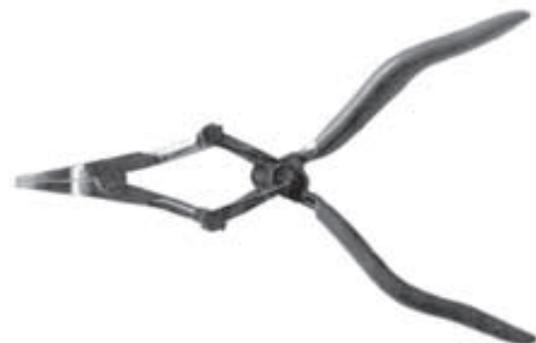
Adjusting pliers to move the segment nut
