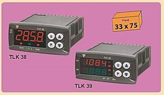
Autotuned, microprocessor based digital controller with 2-, 3-point or PID control and adjustable set point gradient (ramp function)
