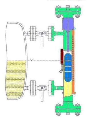
The bypass tube is connected by side / side, or top and bottom connections with the tank. A magnetic float inside the bypass tube rides on the same level as in the tank and operates the coloured flags, the limit switches and / or the optional level transmitter on the outside of the tube.
